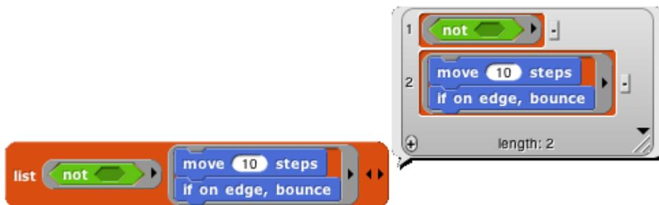
Here, we are making a list of procedures. But the **list** block accepts inputs of any type, so its input slots are not ringed. We must say explicitly that we want the block *itself* as the input, rather than whatever value would result from evaluating the block.
